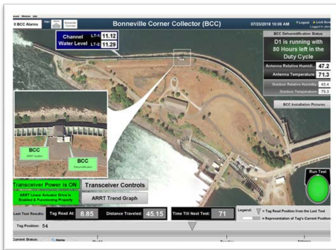
Figures 24 & 25. SCADA drill-through interface showing humidity-control automation for large antenna at Bonneville Corner Collector (BCC)
